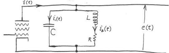
The problem will be solved when we have found e (t). The standard classical procedure would be to set up a differential equation in which e (t) is the unknown and i (t) the driving function. However, in this relatively simple problem, the driving function is not differentiable, and the procedure described would fail.
